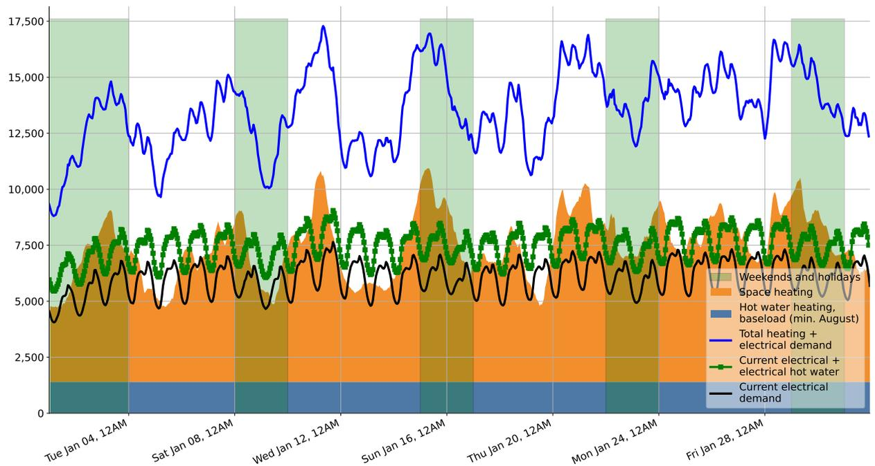
Figure 2: Toronto heat and power demand, January 2022. Heating demand (orange area) is a function of outdoor temperature and wind, and is on a different cycle than electrical demand. Data sources: Environment and Climate Change Canada “Hourly Data Report for January 2022”; IESO “Hourly Zonal Demand Report”; Statistics Canada “Census Profile, 2016 Census, Ontario”; SE Aplin EmissionTrak™ “Residential space heating demand, Ontario.”
