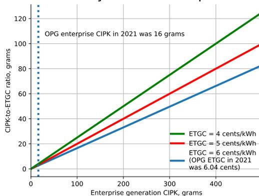
Figure 3: Multiply C-tax rate per gram by CIPK-ETGC ratio to determine C-tax impact on ETGC. OPG data from OPG MD&A, Dec 2021.
